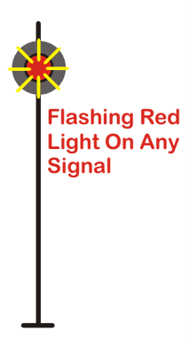
RULE 245N Flashing Stop & Proc
